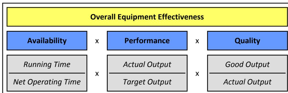
Fig 1: The OEE Calculation and constituent elements<sup>1</sup>.
