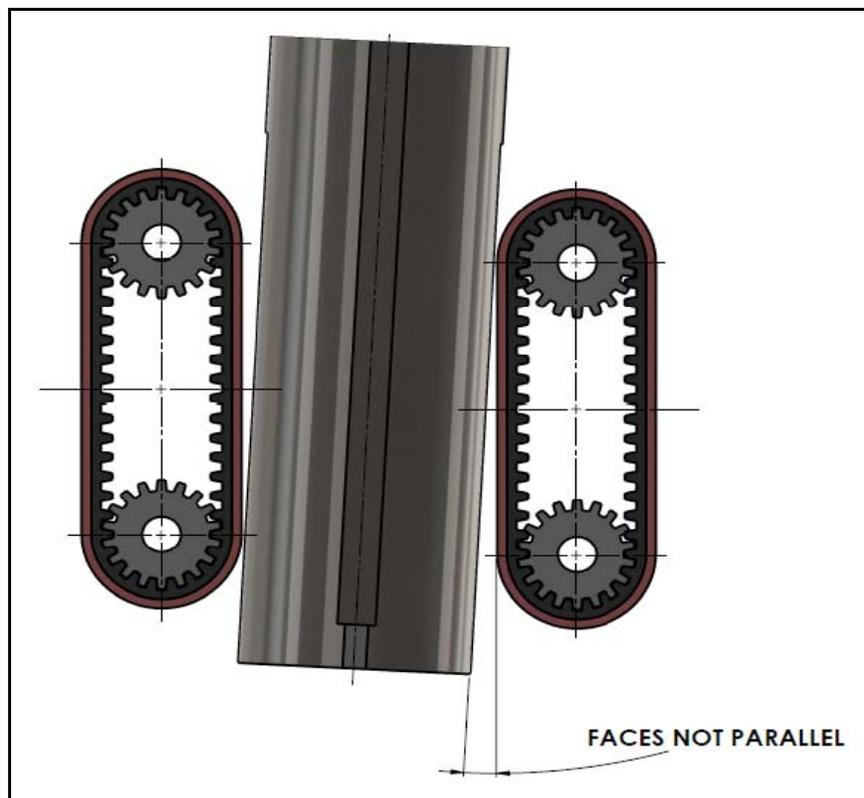
**Fig 3:** Example of tube misalignment.
