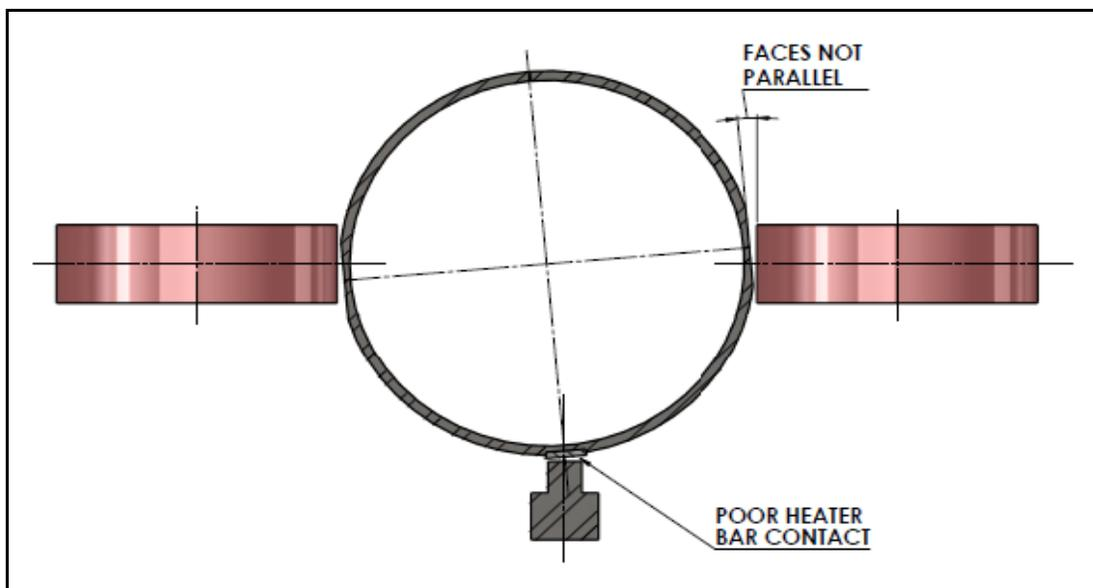
**Fig 4:** Example of tube twist.
