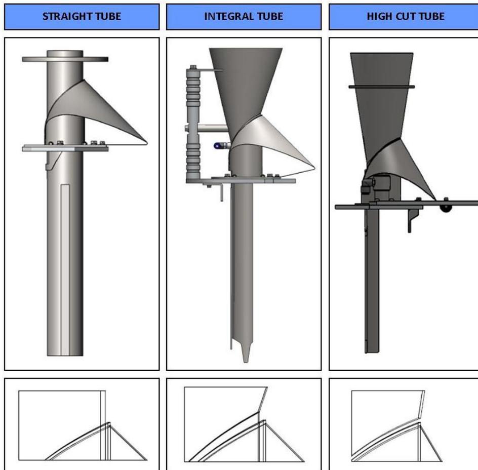
**Fig 2:** Various tube inlet design options.
