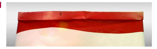
A tear notch makes packages produced on vertical form/fill/seal baggers easier to open. This small slit in the end seal allows consumers to easily tear the film in order to gain access to the product.
