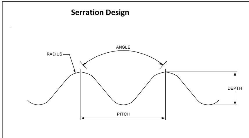
Package design will also have an impact on the application of pressure, as the extra layers of film created by fin seals, lap seals, gussets and folds may produce an uneven pressure distribution across the width of the end seal. Serration design is the primary tool used to overcome difficulties in these situations, with designs specifically engineered to compensate for the varying film thickness.
